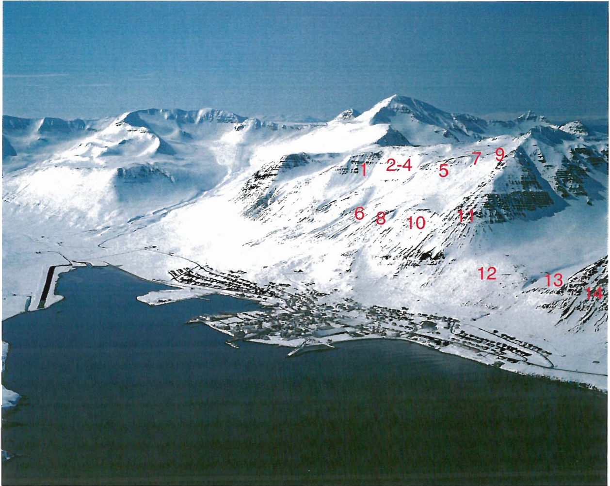
Figure 3. View from north east of the avalanche paths above Siglufjörður. The red numbers indicate the approximate location of starting areas that were delineated during field investigation (see Map 4) (Photo: Mats Wibe Lund).
