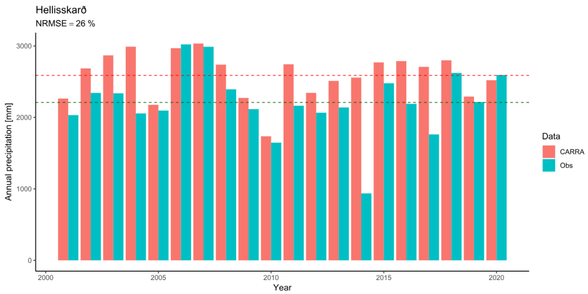
Figure IV.117 — Comparison between the observed and simulated (CARRA) accumulated annual precipitation at the Hellisskarð automatic station.
