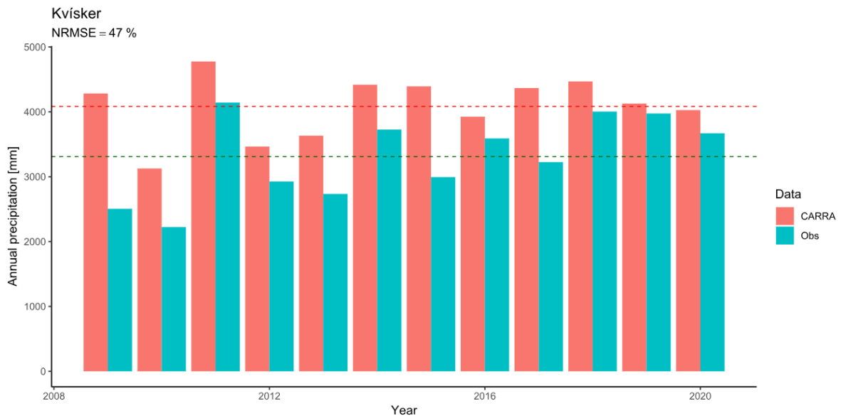
Figure IV.126 — Comparison between the observed and simulated (CARRA) accumulated annual precipitation at the Kvisker automatic station.
