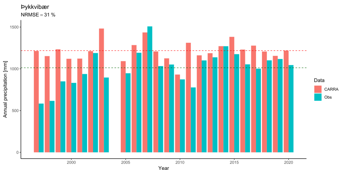
Figure IV.146 — Comparison between the observed and simulated (CARRA) accumulated annual precipitation at the Þykkvibær automatic station.
