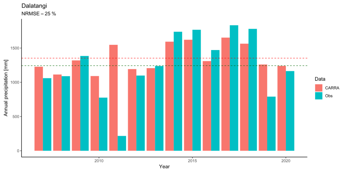
Figure III.106 — Comparison between the observed and simulated (CARRA) accumulated annual precipitation at the Dalatangi automatic station.
