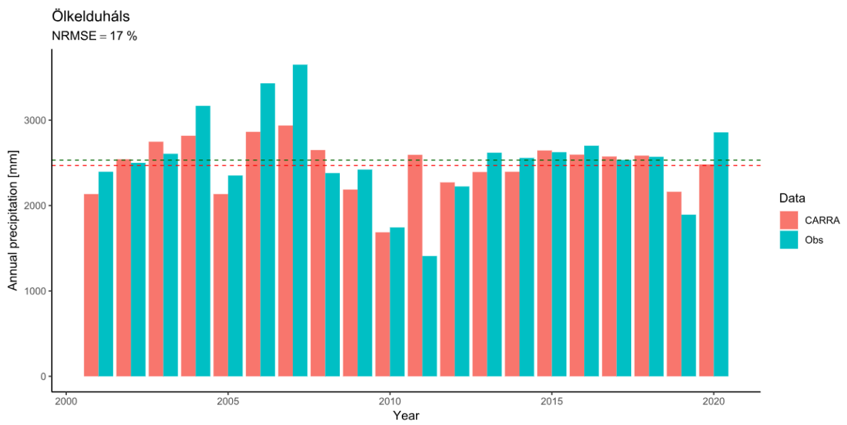
Figure IV.147 — Comparison between the observed and simulated (CARRA) accumulated annual precipitation at the Ölkelduháls automatic station.
