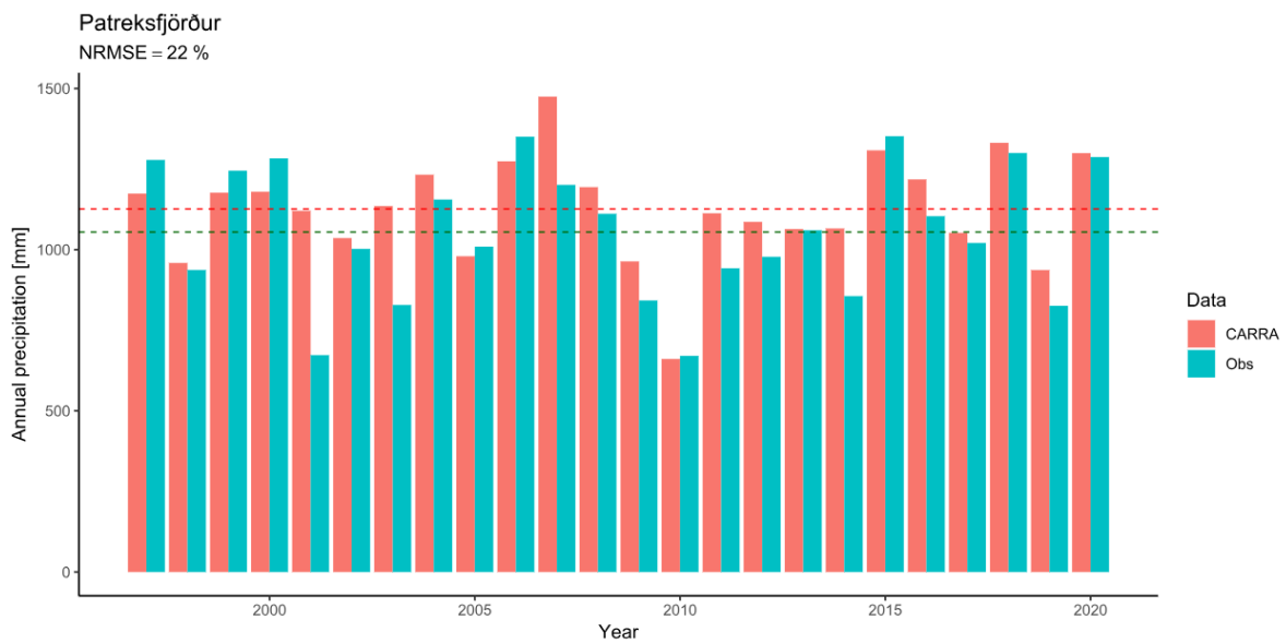
Figure IV.133 — Comparison between the observed and simulated (CARRA) accumulated annual precipitation at the Patreksfjörður automatic station.
