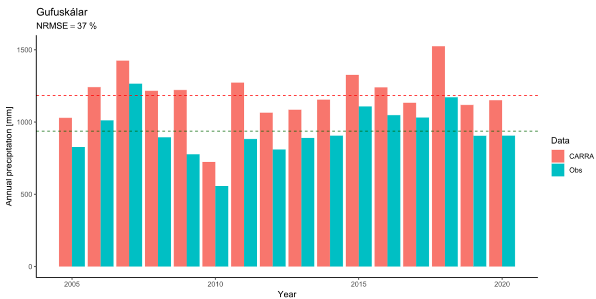
Figure IV.114 — Comparison between the observed and simulated (CARRA) accumulated annual precipitation at the Gufuskálar automatic station.
