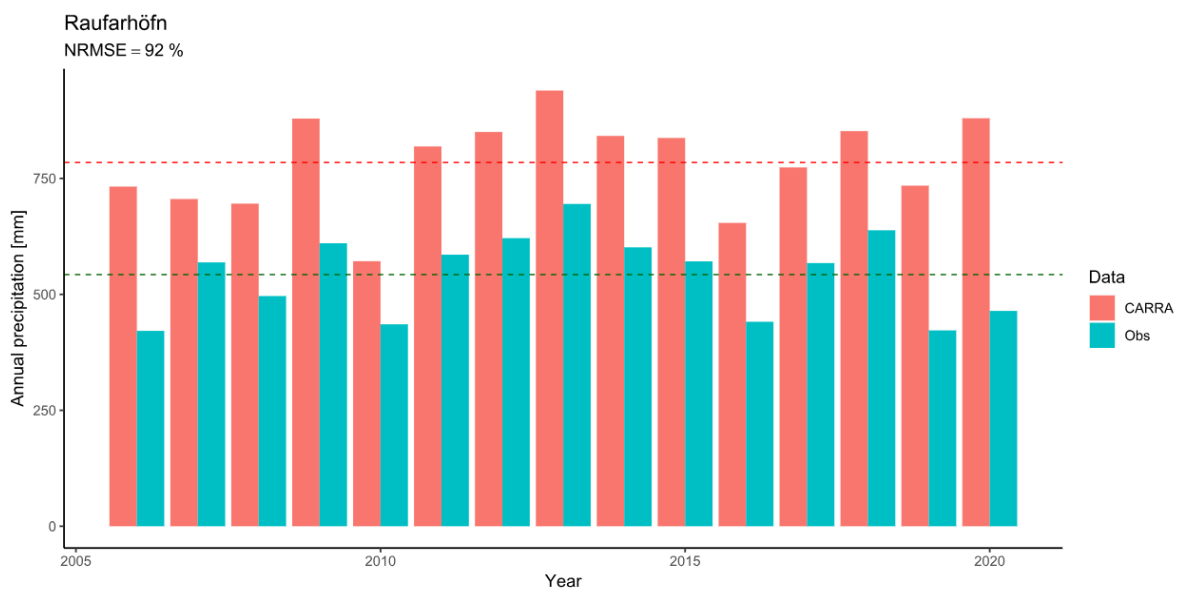
Figure IV.134 — Comparison between the observed and simulated (CARRA) accumulated annual precipitation at the Raufarhöfn automatic station.
