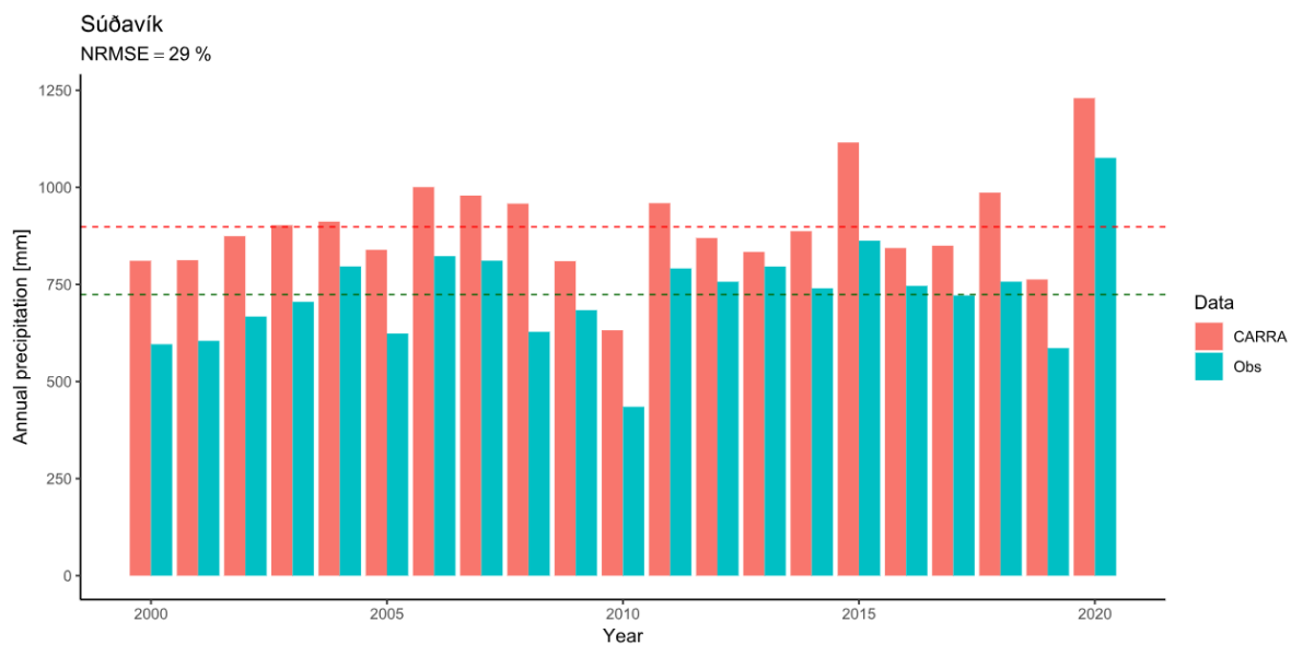
Figure IV.141 — Comparison between the observed and simulated (CARRA) accumulated annual precipitation at the Súðavík automatic station.
