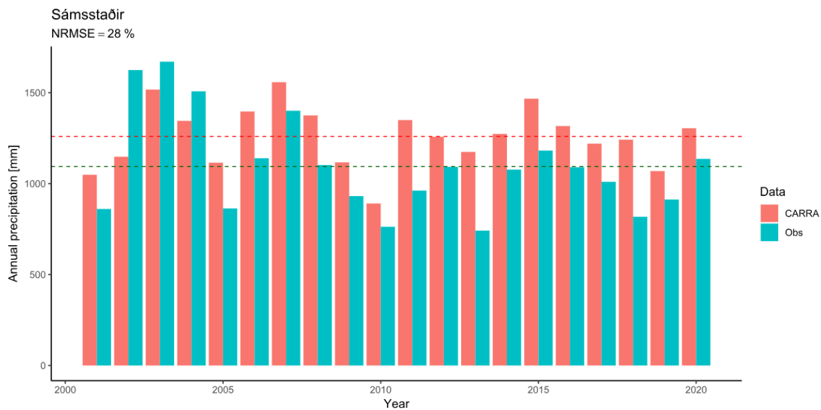
Figure IV.137 — Comparison between the observed and simulated (CARRA) accumulated annual precipitation at the Sámsstaðir automatic station.
