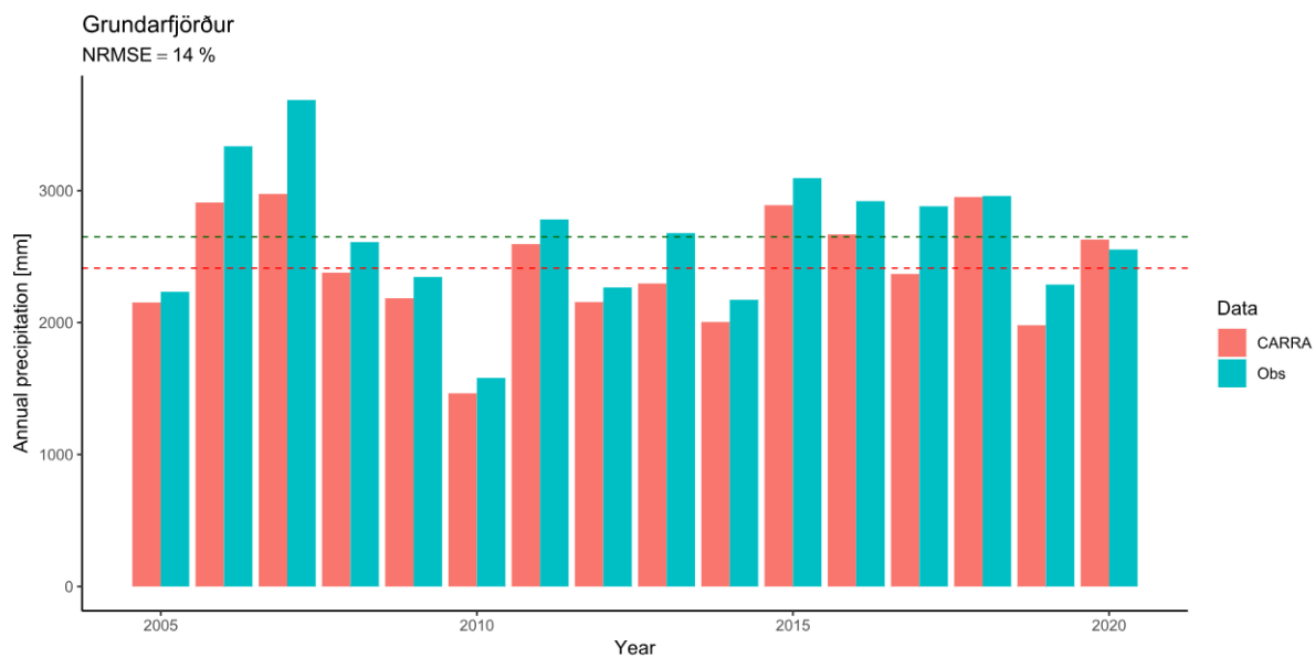
Figure IV.113 — Comparison between the observed and simulated (CARRA) accumulated annual precipitation at the Grundarfjörður automatic station.
