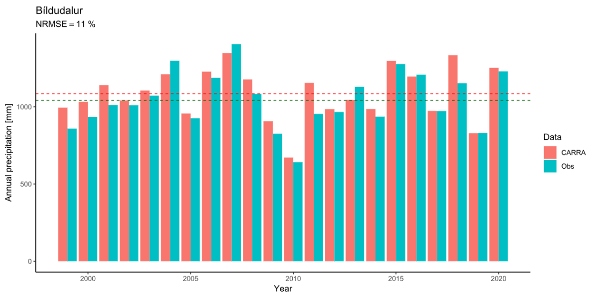
Figure IV. 100 — Comparison between the observed and simulated (CARRA) accumulated annual precipitation at the Bíldudalur automatic station.
