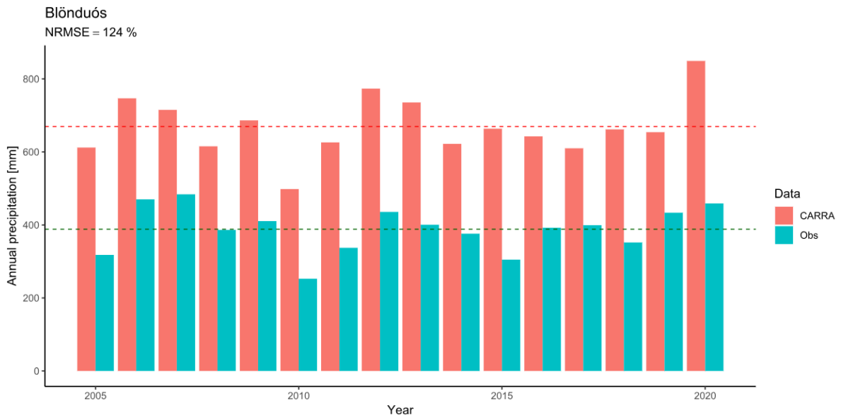
Figure IV.101 — Comparison between the observed and simulated (CARRA) accumulated annual precipitation at the Blönduós automatic station.
