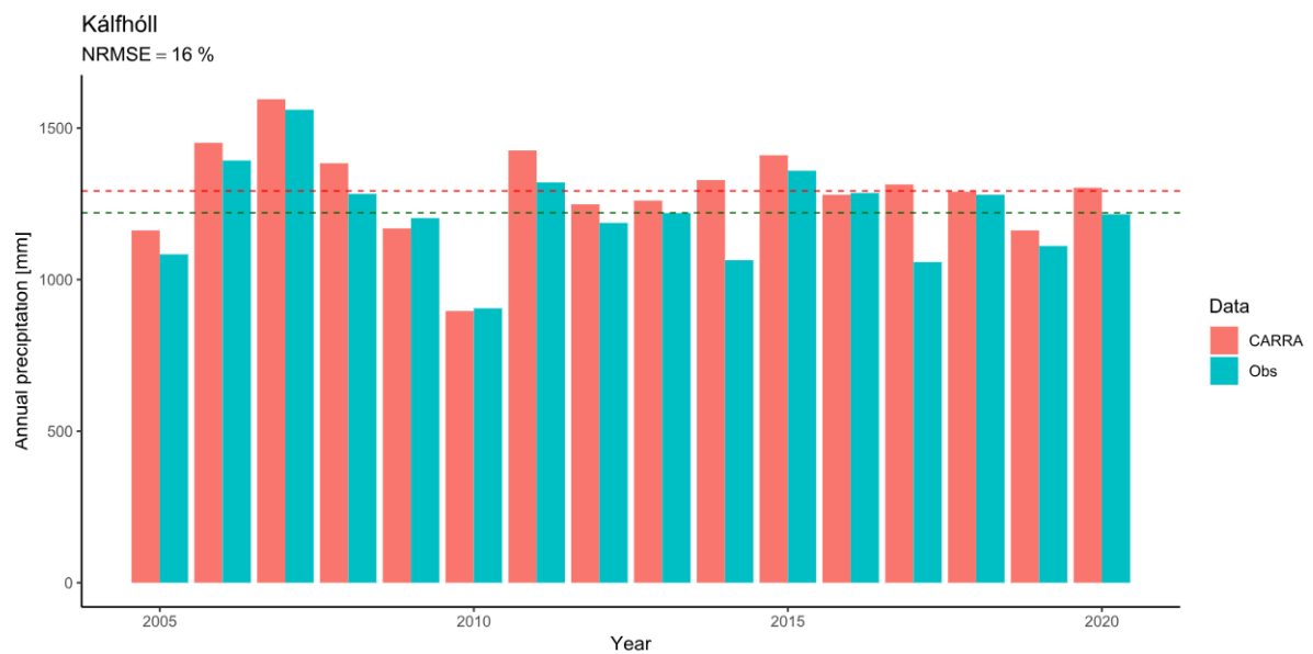
Figure IV.122 – Comparison between the observed and simulated (CARRA) accumulated annual precipitation at the Kálfhóll automatic station.
