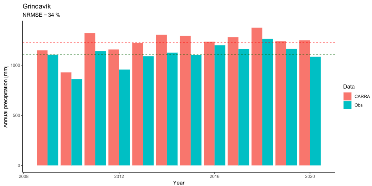
Figure IV.112 — Comparison between the observed and simulated (CARRA) accumulated annual precipitation at the Grindavík automatic station.
