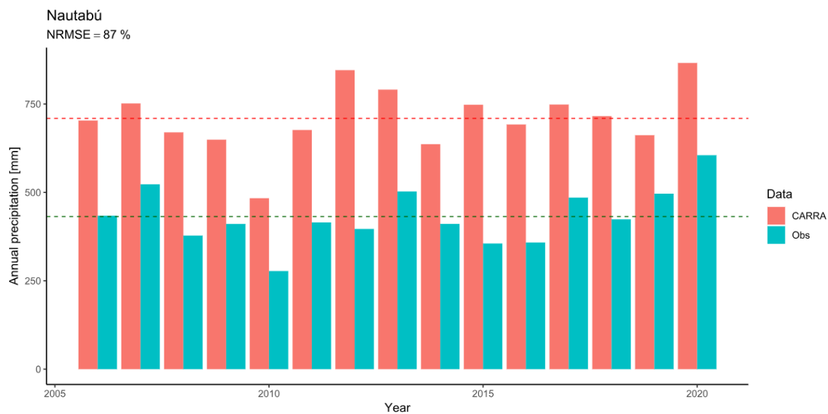
Figure IV.129 — Comparison between the observed and simulated (CARRA) accumulated annual precipitation at the Nautabú automatic station.
