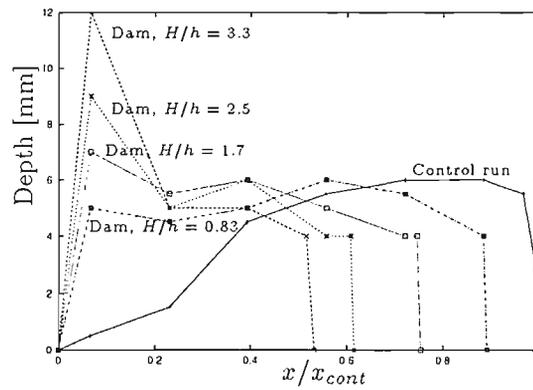
Figure 46: Averaged length profile for the dams.
