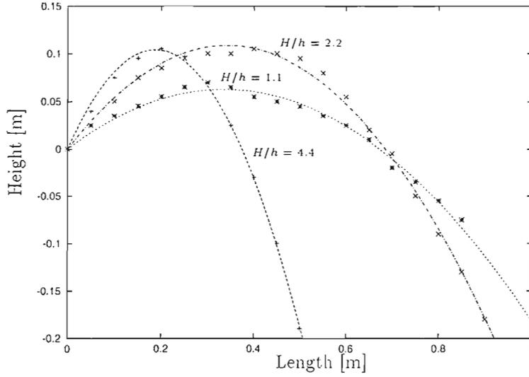
Figure 10: Jet profiles for 2.5, 5.0 and 10.0 cm high dams.
