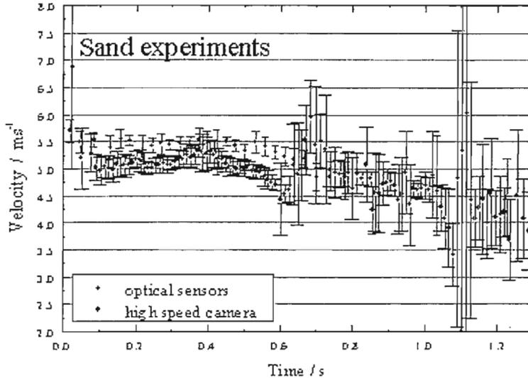
Figure 20: Velocity at the sliding surface of the chute compared to the surface velocity for the sand experiments.
