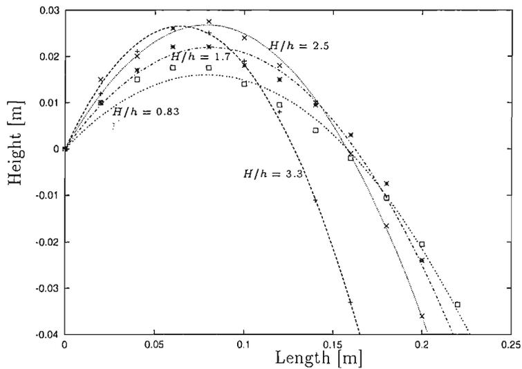
Figure 31: Jet profiles for 0.5, 1.0, 1.5 and 2.0 cm high dams.
