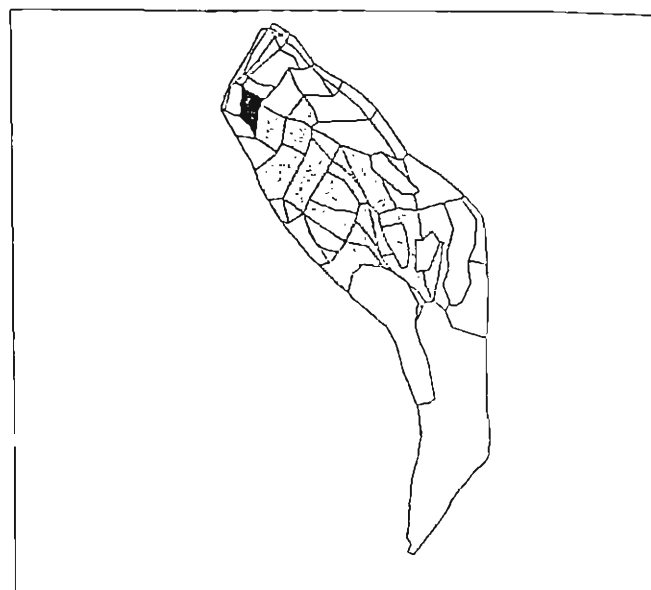
Fig. 8. An example of release in the Drayre avalanche path. The panel in black is considered to be the trigger. The shaded panels are considered to be released.
