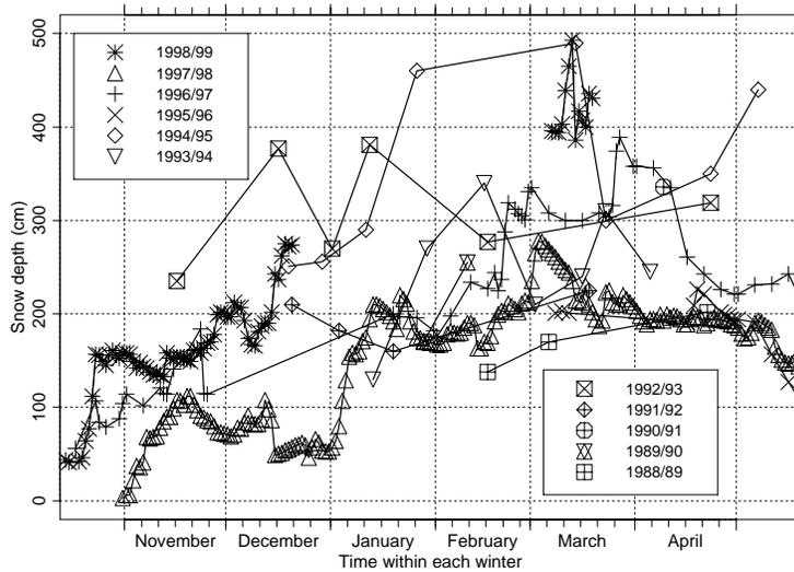
**Figure 2.** Snow depth at the stake *isse00* at 576 m a.s.l. in Seljalandshlíð above Seljalandsdalur. Data points, where the snow depth at buried stakes has been inferred, based on the measured variation of the snow depth at other nearby stakes, are denoted with a circle.
