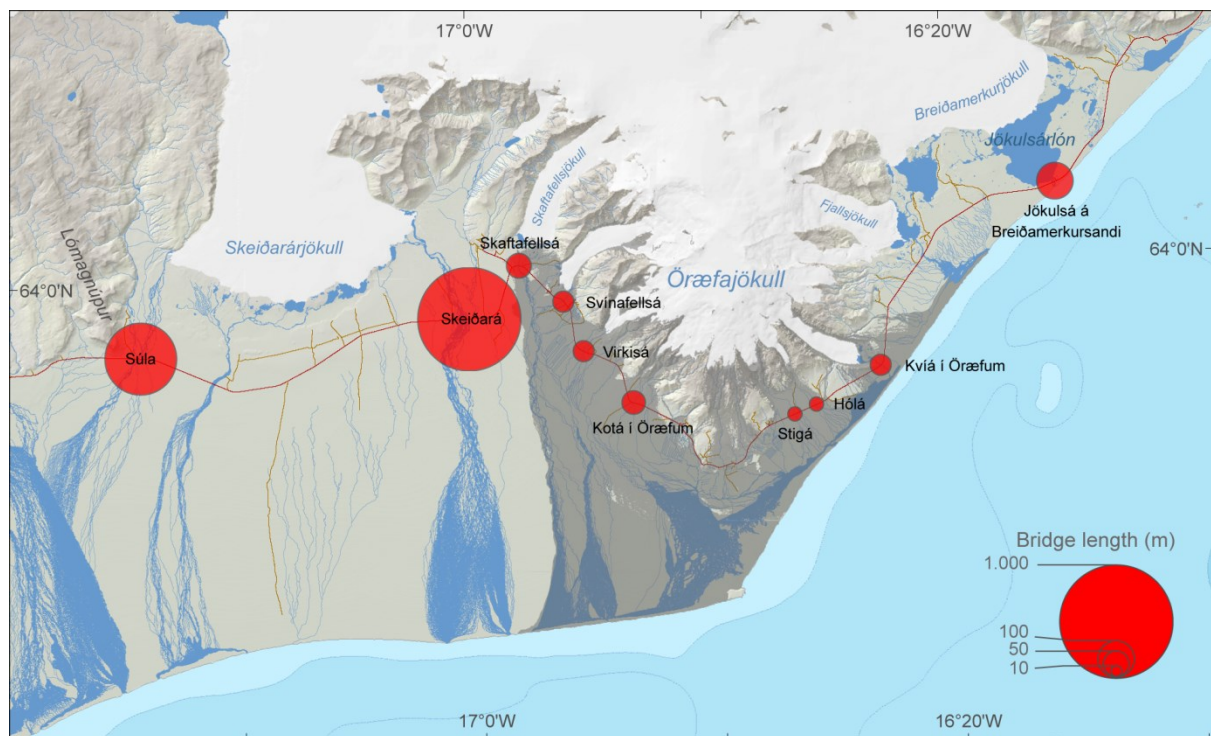
Figure VII-17: Single-lane bridges (red-filled circles) located on the Lómagnúpur - Jökulsárlón National road's segment (Source: IRCA, 2011). Seven bridges are located in the area identified at risk of volcanogenic floods (grey area) by Helgadóttir et al. (2015).
